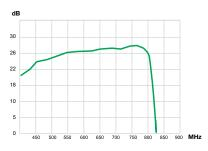
Canaux: 21-60 UHF Rapport Av/Ar: >15 dB Alimentation: 5-24V DC Montage sur mât Ø 25-45mm Dimensions: 320 x 350 x 150mm
