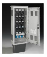
LV panels ensuring and guaranteeing high breaking capacity fuse protection for network conductors and transformers on a pole from 50 to 160 kVA and up to 400 kVA. For public distribution overhead LV networks. Four-pole distribution panels with neutral conductor insulation and distribution.
