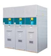
Full range of air insulated switchgear modular distribution units of up to 36 kV in a metal enclosure, equipped with a breaker, switcher, disconnecter and fuses.
